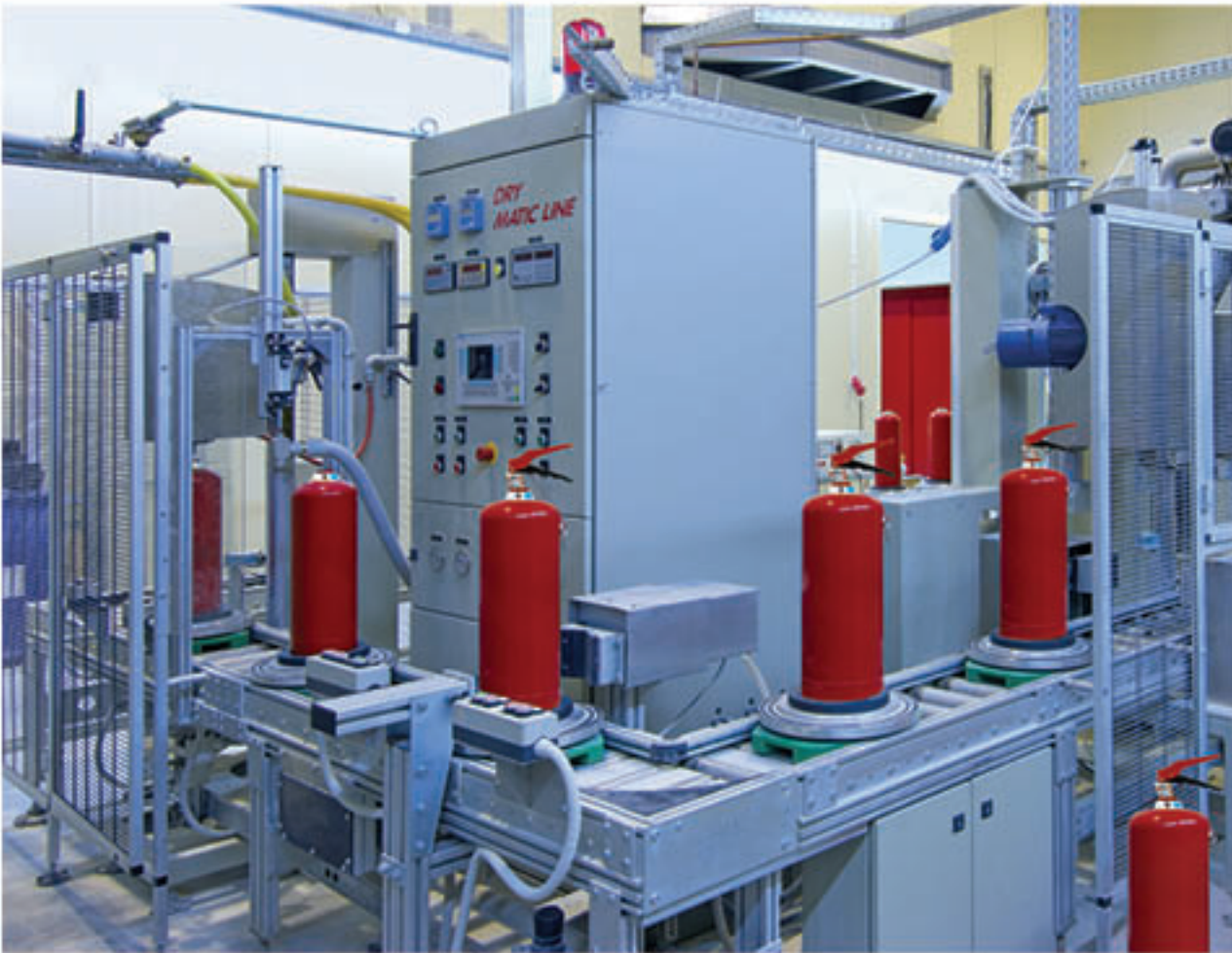
Manufacturing Procedure in Stages: - Automatic Filling Procedure of Dry Powder / Foam / ABF-Wet Chemical Extinguishers
