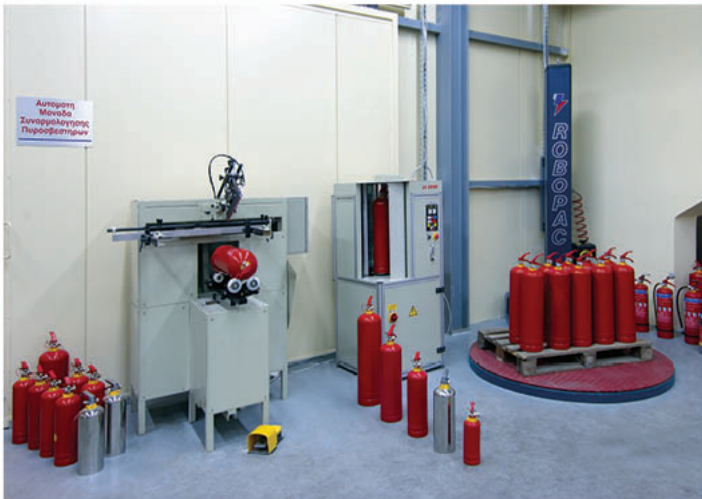
Silk Screening Machine Silk Screening Unit is used for Fadeless Printing Fire Extinguishers
