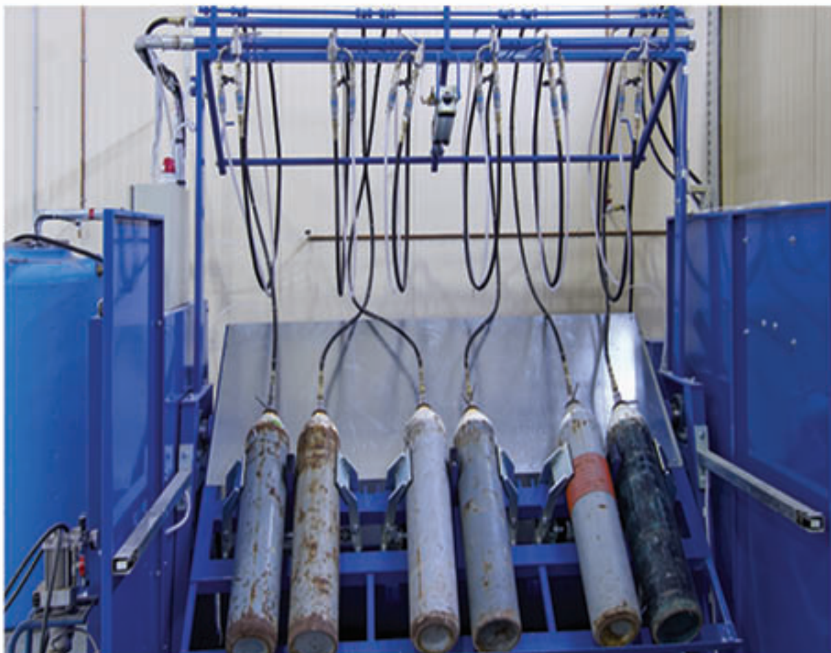
Hydraulic 6-Position Testing Machine for Gas and Fire Extinguisher Maximum Production Capacity of 30 Cylinders per Hour - Maximum Test Pressure 450bar
