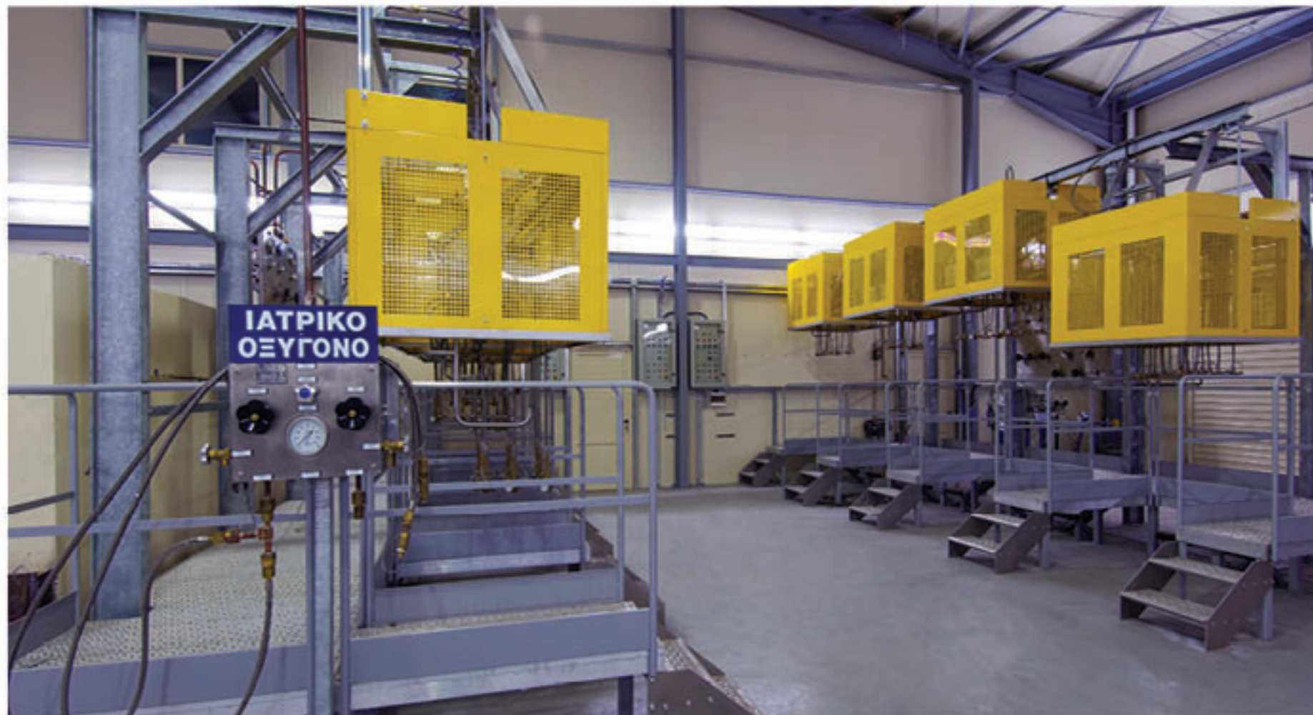
Automatic Gas Bottling Unit (Medical and Industrial Oxygen, Nitrogen, Argon, CO 2 , Mixtures e.g. IG 541, IG 55, Banarg etc.)
